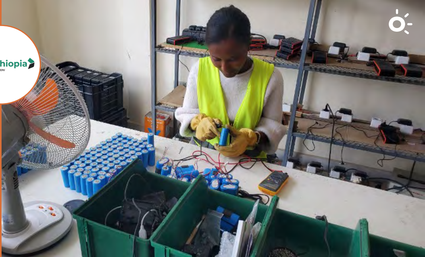
IES battery technician collecting, sorting, and physically checking cells from a dismantled used battery in the IES warehouse, Addis Ababa, Ethiopia (2026)
