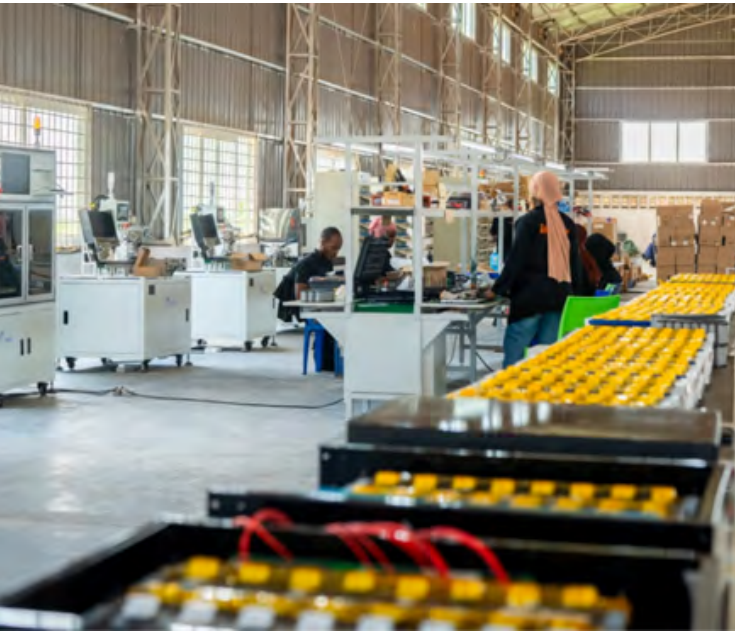
Cylindrical and prismatic cell pack assembly lines, Kirolo production facility (2025)
