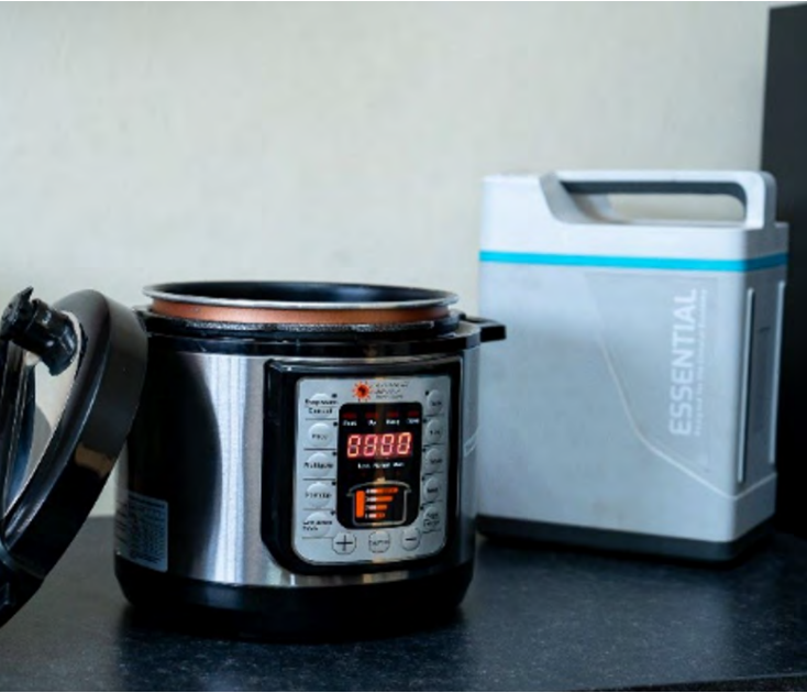
AceleAfrica's second-life lithium-ion battery powering an electric pressure cooker in Nairobi, Kenya (2026).
