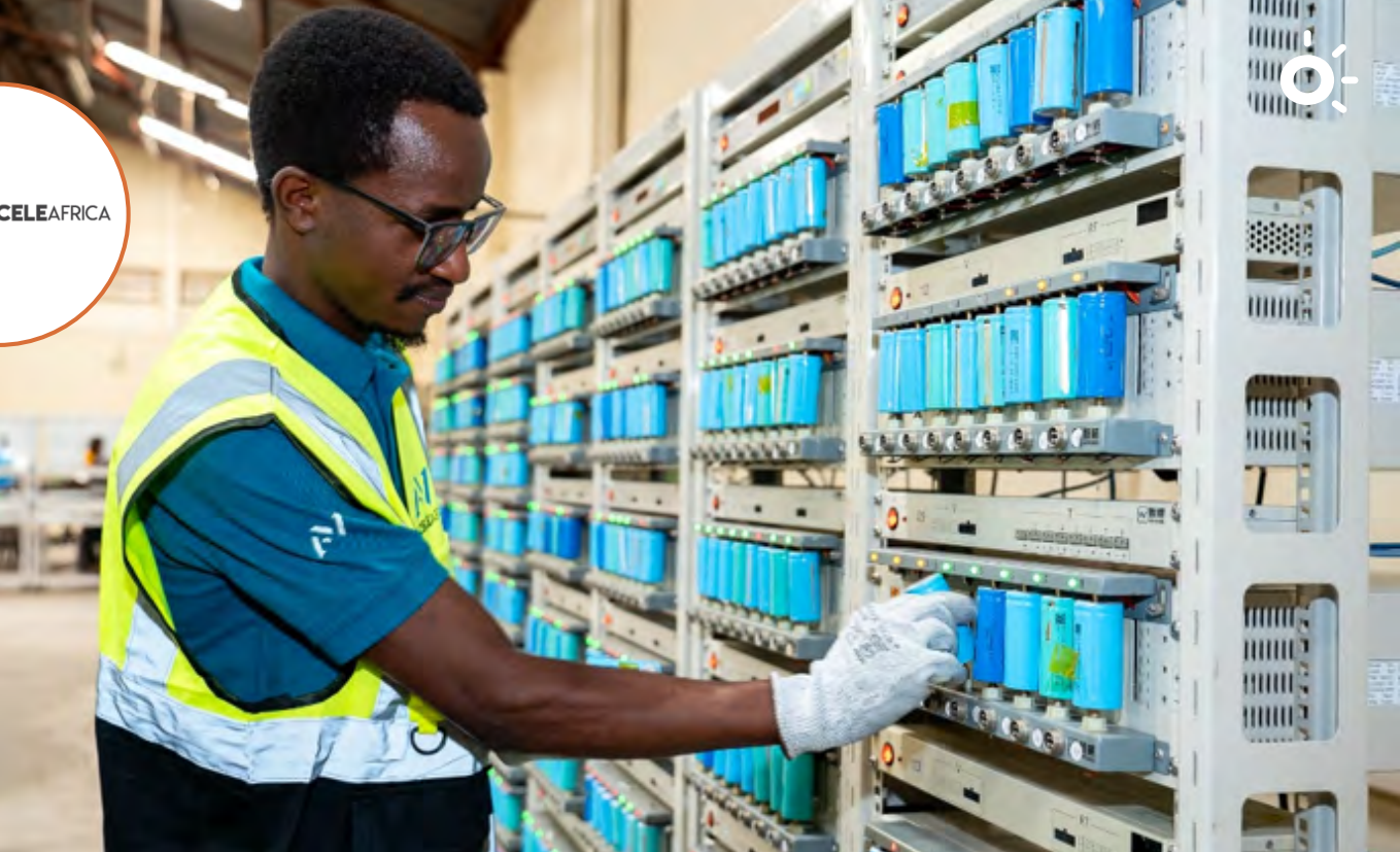
Used Lithium-ion cell testing and grading machines at AceleAfrica’s workshop in Nairobi, Kenya (2026).
