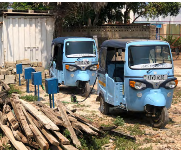
Figure 12 – CHAJI provides the only public charging available for e-tuktuks in Mombasa, Kenya. Source: CHAJI.
