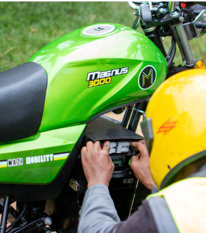
Image: Mazi rider fixes the battery connector during a swap, ensuring a secure connection for smooth and reliable electric mobility. Mazi Mobility. Nairobi, Kenya, 2023.
